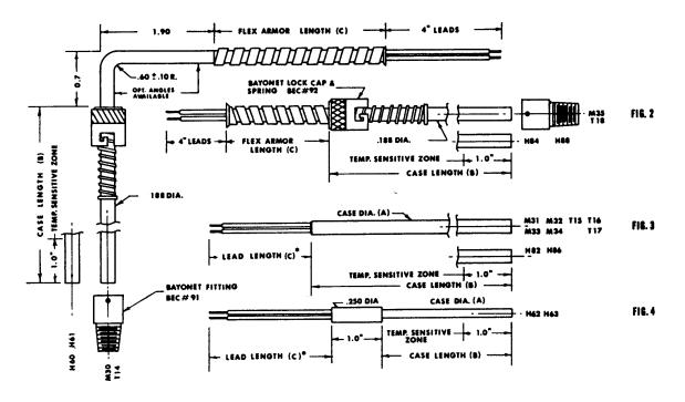
\*LEAD LENGTH (C) AVAILABLE AS LEAD WIRE, FLEXIBLE ARMOR, STAINLESS STEEL OR COPPER BRAID
