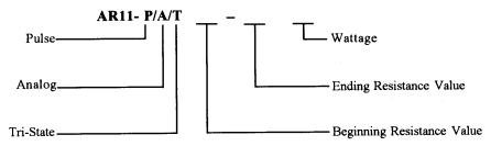
\* If you need a resistance range that cannot be met by one of the Resistor Networks at the end of the Specification section, you must also supply wattage and tolerance of the RN. Please specify with 1/4 watt 1% or 1/2 watt 5% resistances if possible. Custom wattages and tolerances may increase cost and lead times.
